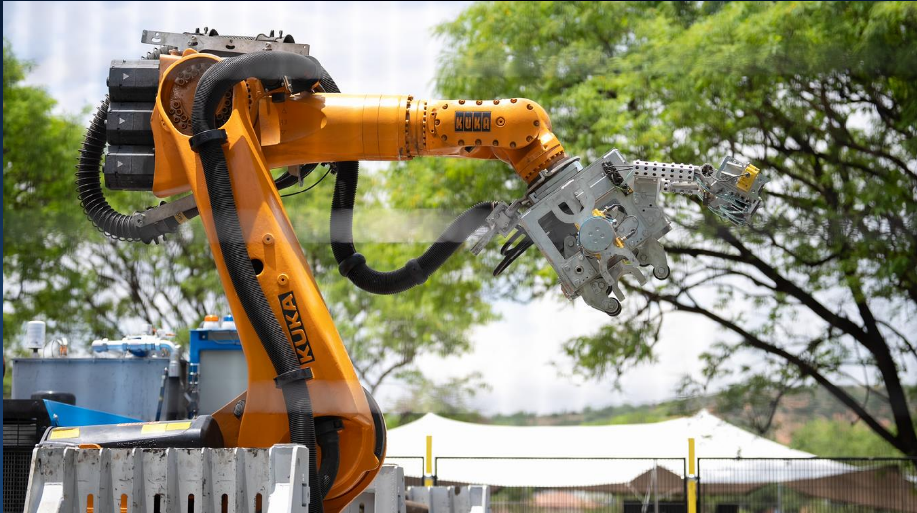
Image: Desert Elephant surface robotic core drilling rig.
