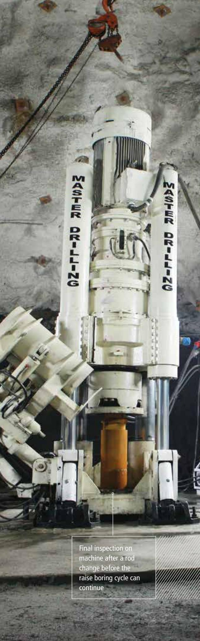
Final inspection on machine after a rod change before the raise boring cycle can continue
