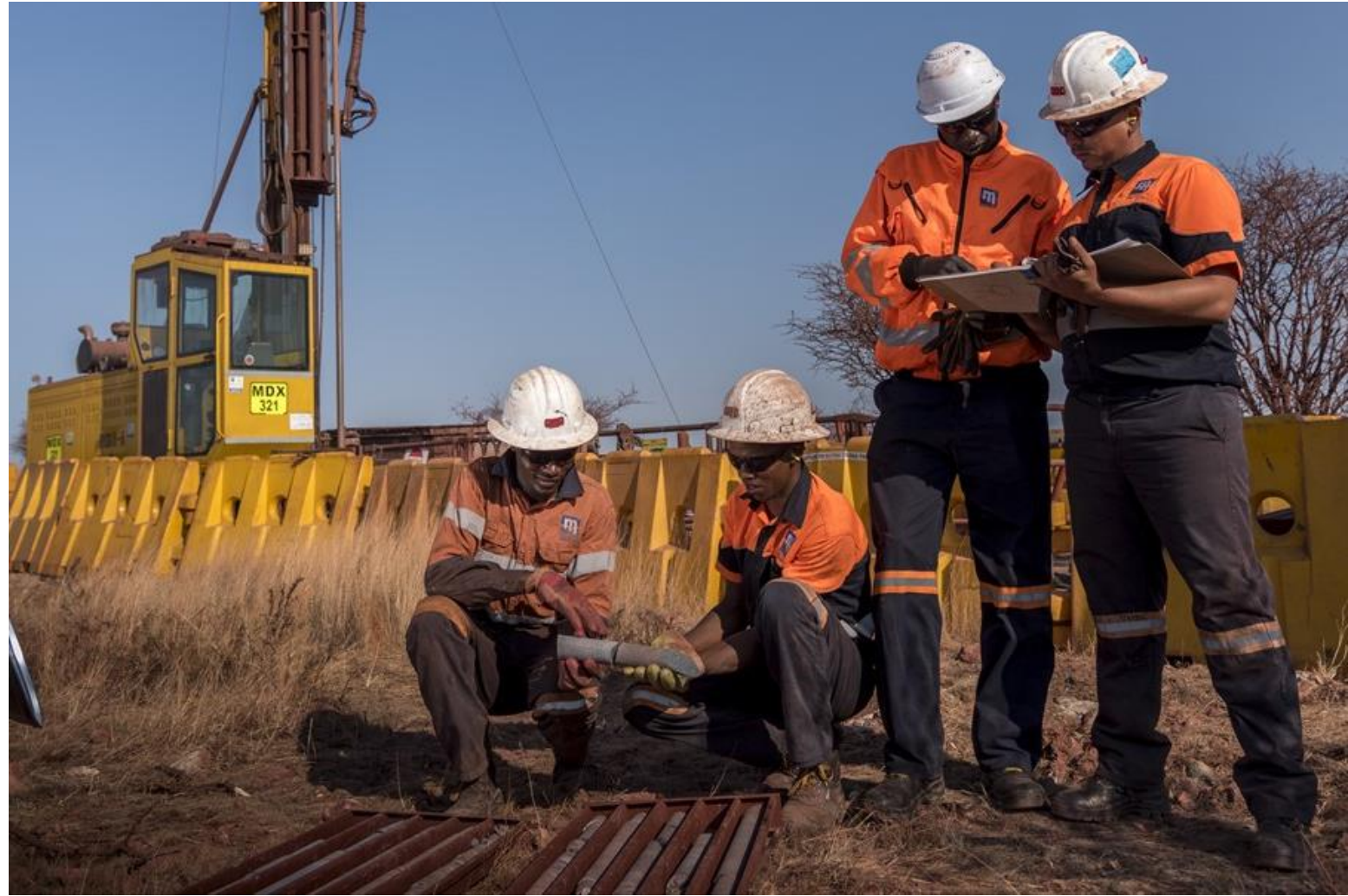
Image: Core logging by field geologists at Kolomela Mine
