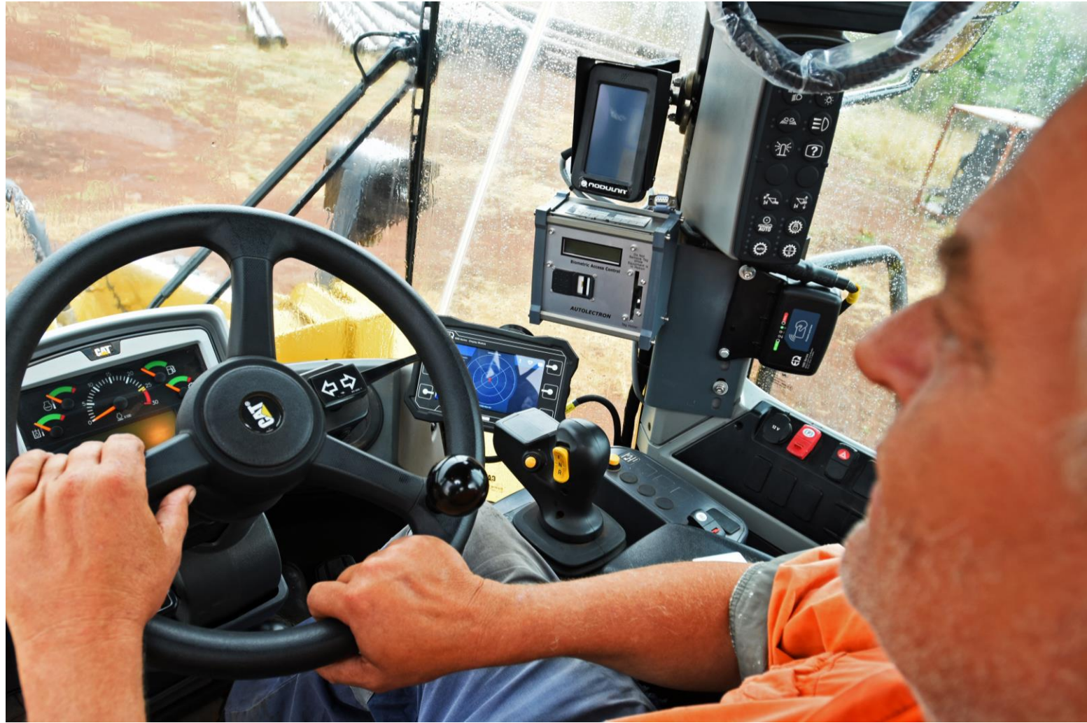
Image: An A&R proximity detection device fitted to a Wheel Loader onsite
