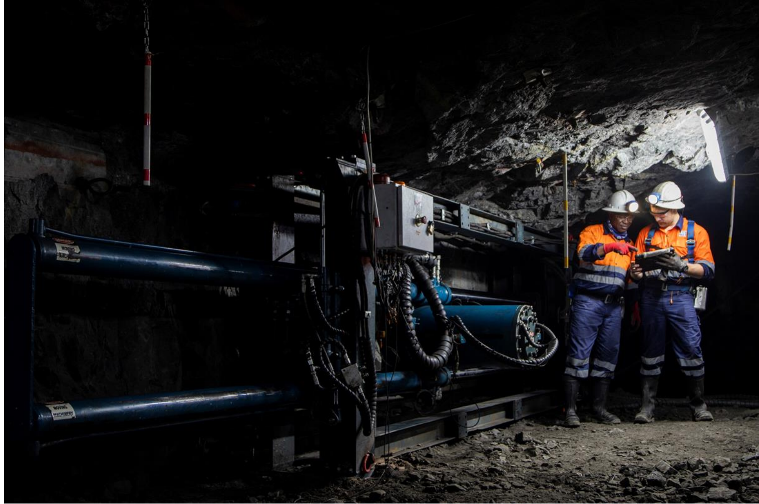
Image: Experimental Rock Cutter testing for the ARM project on the PGM Reef underground
