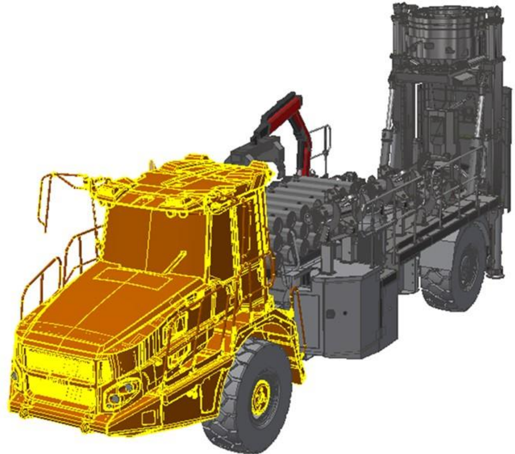
Image: CAD model of the LP100 Raise Boring machine
